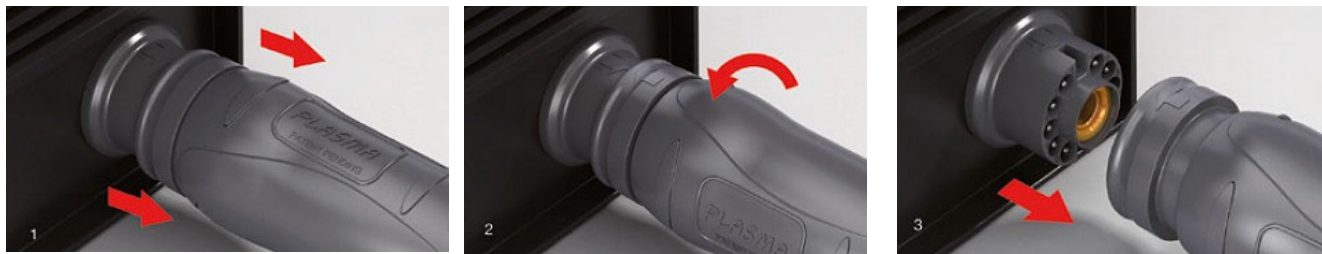
Fig.4-3: Disconnect the torch connection
