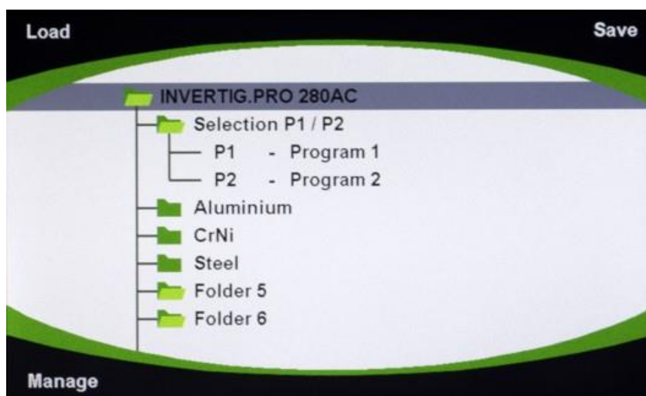
Fig. 24: INVERTIG.PRO digital / Programs application (Progr.) control panel
