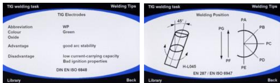
Fig. 42: INVERTIG.PRO digital / Assist application control panel Library view WIG electrodes and welding position
