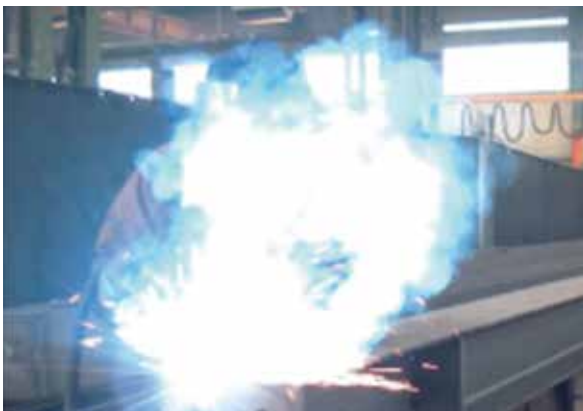
Previously: Severe smoke development with conventional arc.
