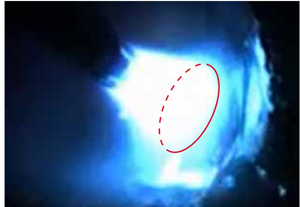
Now: FOCUS.ARC Concentrated arc with centered energy
