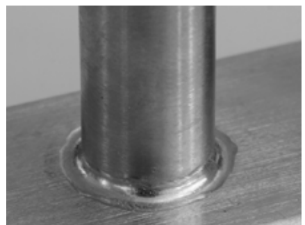
■ Circumferential weld Function: HYPER.PULS without filler material
