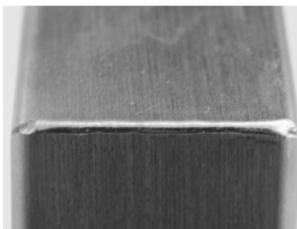
■ Corner weld Function: HYPER.PULS with filler material
