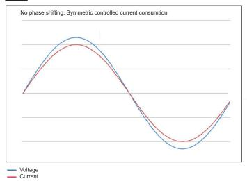
A PFC is able to correct the phase shifting as well as the peaks from the current.
