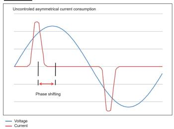
Primary inverters are for the power supply network a capacitive load. This generates a phase shifting between current and voltage. The result is reactive power.
