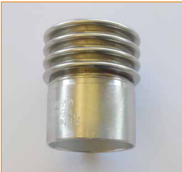
Circumferential welding | hand-held torch (3.0 mm on 0.2 mm)
