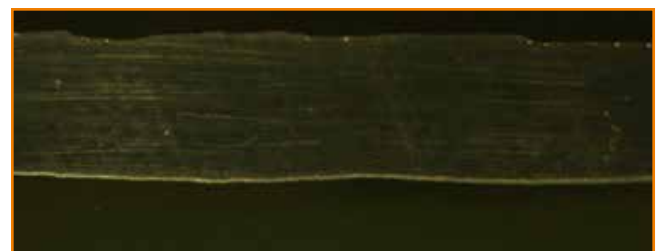
Repair welding with DualWave. Far fewer pores.
