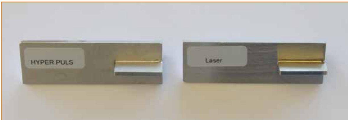
Corner weld for pharmaceutical engineering | without filler, hand-held torch
