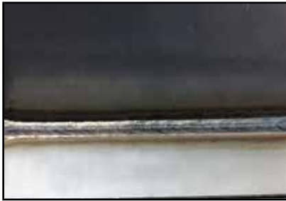
■ CrNi fillet weld PB | 1.0 mm POWER.ARC
