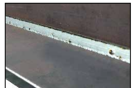
■ Steel fillet weld PB | 10.0 mm FOCUS.ARC
