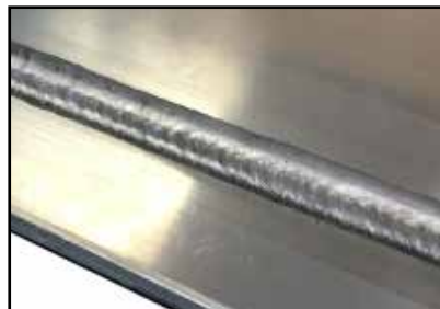
■ Aluminium fillet weld PB 5.0 mm | POWER.PULS
