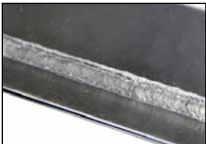
■ Aluminium fillet weld PB 1.5 mm | POWER.ARC
