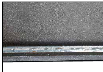
■ Steel fillet weld PB | 5.0 mm POWER.PULS
