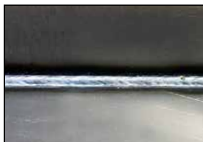
■ Steel fillet weld PB | 2.0 mm POWER.PULS
