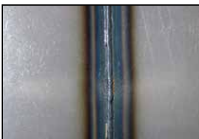
■ Steel butt weld PG | 2.0 mm FOCUS.ROOT
