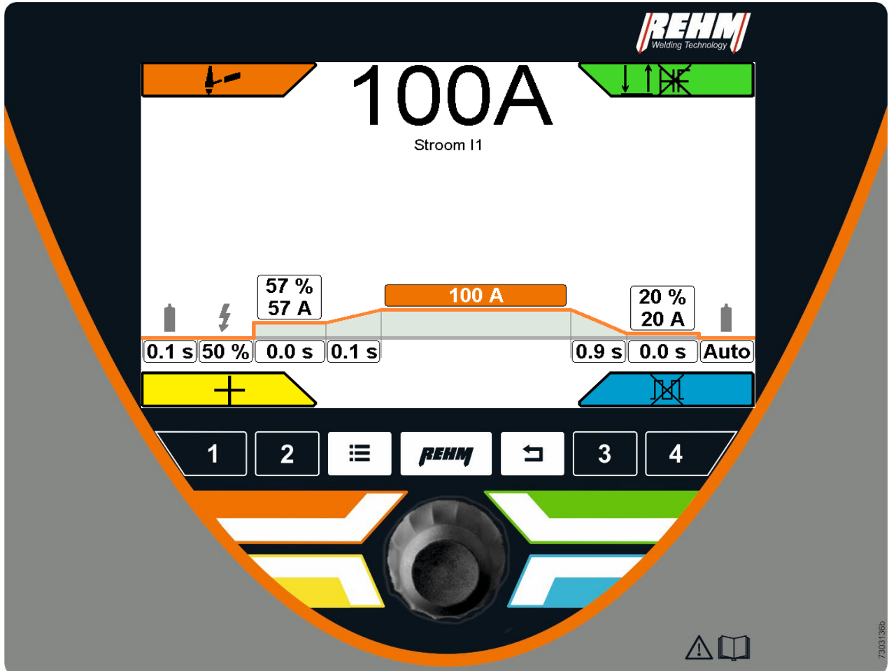
Figure 5: INVERTIG 450 i operating elements and main screen
